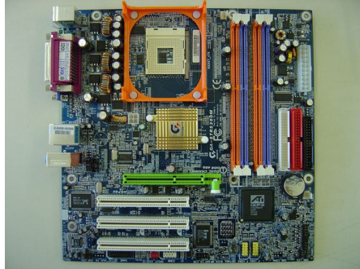
831.000.019 PC Motherboard Gigabyte micro ATX Charge GA8TRS300M (orange CPU socket): BIOS 49 from system 309 (SB V10.00) Charge GA-8TRS350 (yellow CPU socket): BIOS 52 from system 312 (SB V10.02) Attention: Use only Samsung original Memorys - 831300015 Charge SAMSORIG
