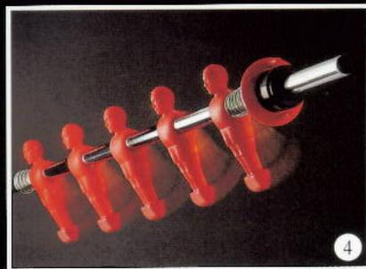
3) Cold drawn steel (25 NC 6) rods (diameter 16 x 2.3 mm<sup>2</sup>) with high stress resistance (R = 100 Kg x mm<sup>2</sup>) and 15 micron thickness chromium plating. One-colour (red-blue) standard players moulded to the bars (on request three-colour selflocking players in red-black-pink and blue-black-pink). Telescopic rods for greater safety also available.
